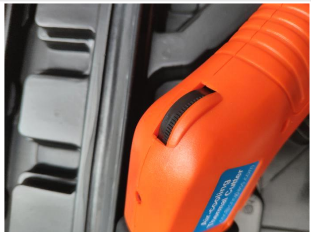
CNC02 air-cooling thermal cutter (16-section dial)
