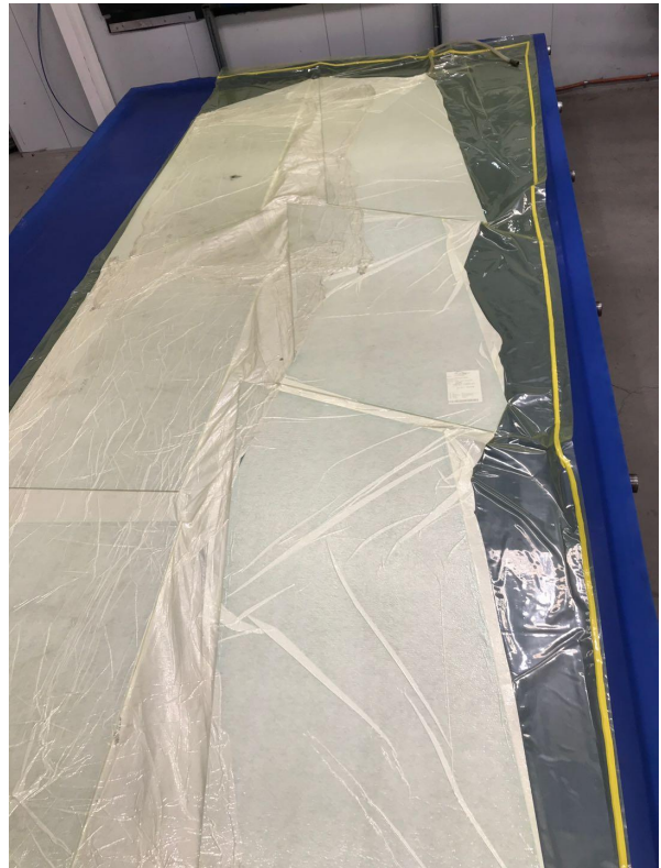
Vacuum bag application — sealant tape edge seal with breather
