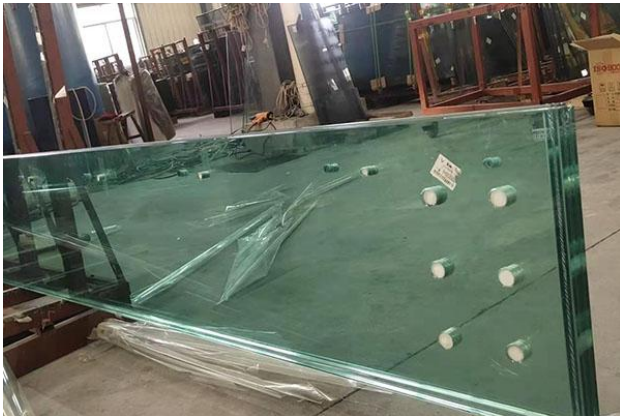
Point-supported facade glass — drilled laminate
