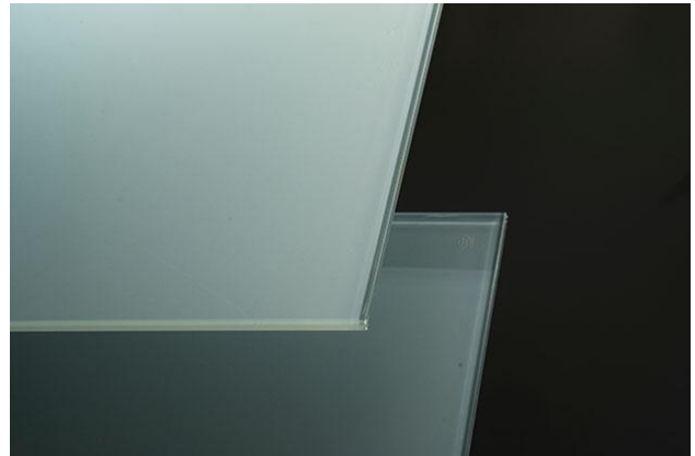
Sandblasting / milky white SGP laminated samples
