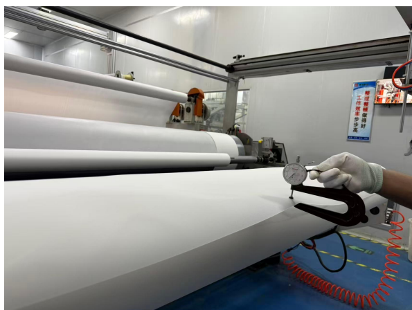
Quality control — thickness measurement on EVA film roll
