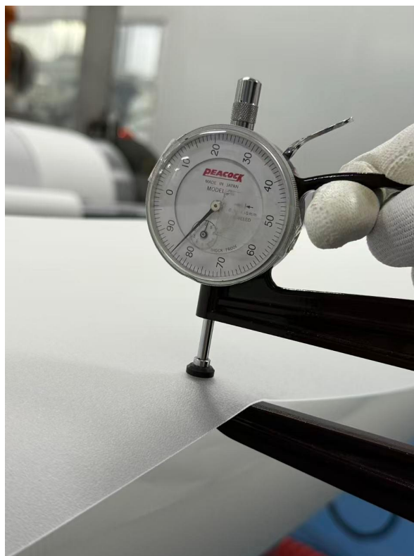
Precision gauge — 0.38 mm film thickness
