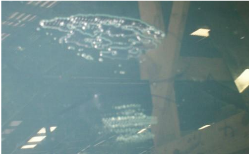
Example: bubble defect in EVA laminated glass (illustrative process photo).
